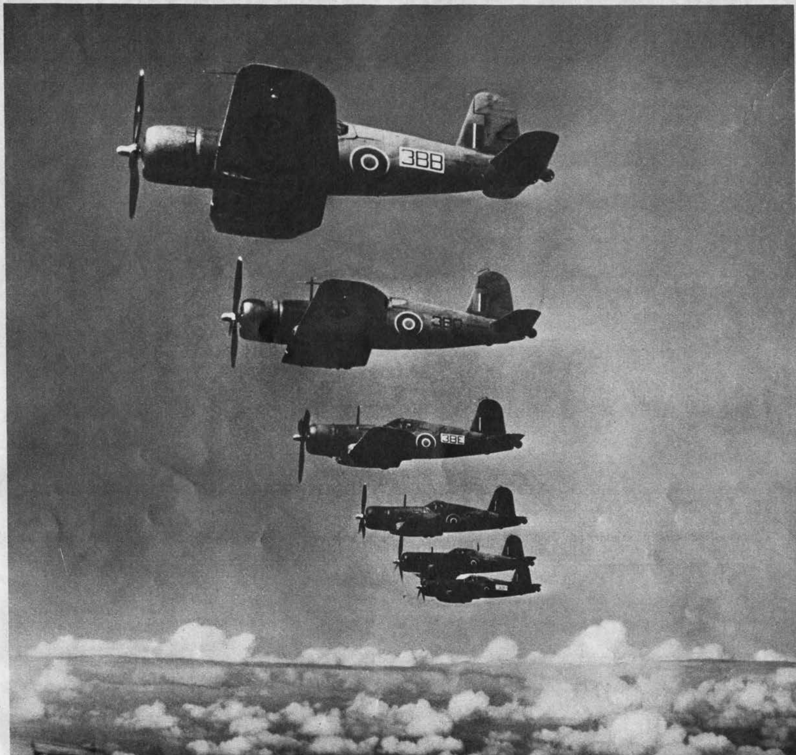
CORSAIR Clipped wingtips distinguish British Corsairs from those flown by U. S. Navy and Marine pilots. Otherwise they are identical and can be recognized by the in-
